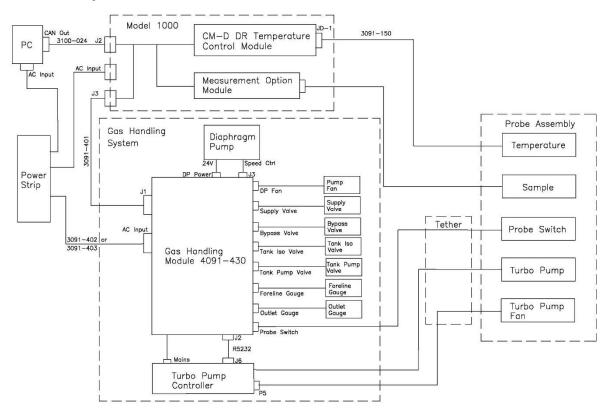
Figure B-1. System cabling/block diagram
