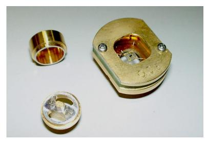
Figure 2-11. DR Heat Capacity Sample Mount and Accessories
