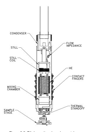
Figure 2-2. Dilution unit and condenser tube
