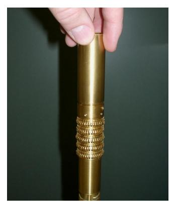
Figure 4-1. The radiation shield unscrews from the condenser tube.
