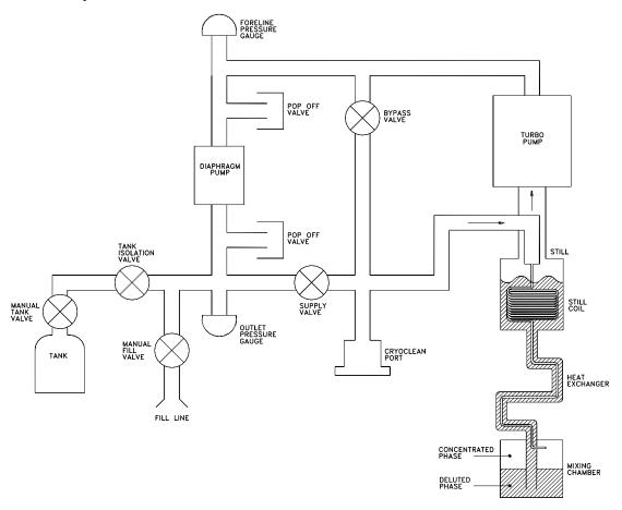
Figure 1-1. Functional diagram of the dilution refrigerator
