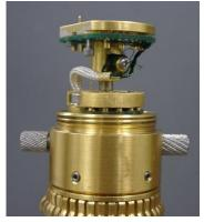
Figure 2-15. Sample mounting pins used to secure the mixing chamber.
