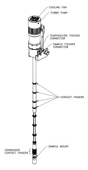
Figure 2-1. Dilution Refrigerator Probe
