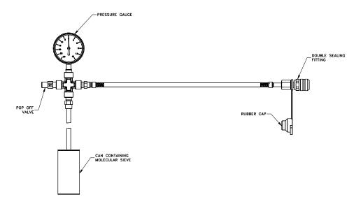
Figure 2-8. Liquid nitrogen cold-trap for DR
