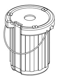
Figure 2-10. Liquid nitrogen dewar flask
