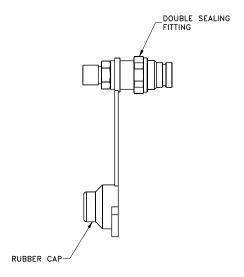
Figure 2-9. Cold-Trap Regeneration Fitting
