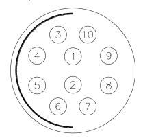
Figure B-2. DR probe connector pin designations
